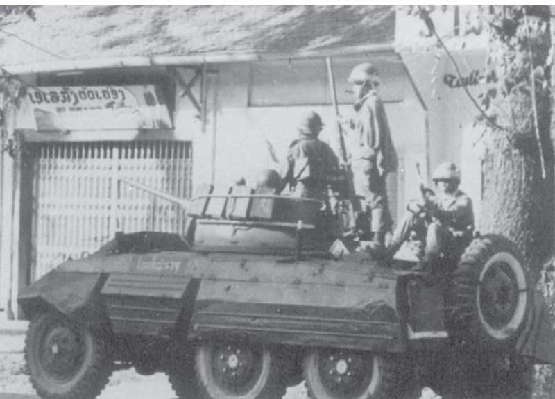
Pro-Kouprasith forces ride on an M-8 Greyhound armored car as they patrol Vientiane after the coup d'état, in February of 1965. The vehicle is armed with a 37mm cannon and a .50 caliber machine gun mounted on the rear of the open turret. (Al Rich Collection, Air America Archives)
