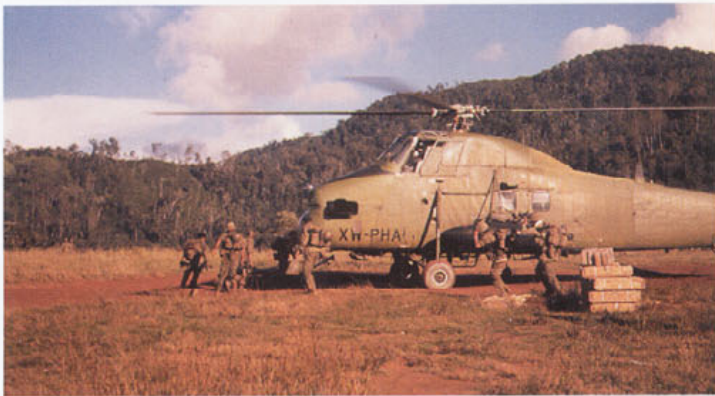
An Air America S-58T Twin Pac (XW-PHA) loads troops and supplies near Pa Doung (Lima Site 5). This helicopter was the first of five Sikorsky H-34s that were converted to turbine engines at Air America's Udorn, Thailand facilities during the Spring of 1971. During their first few months in operation, the S-58Ts were painted in the more traditional Silver and Blue Air America color scheme, but that scheme quickly gave way to overall Olive Drab. (Hugh Tovar)
