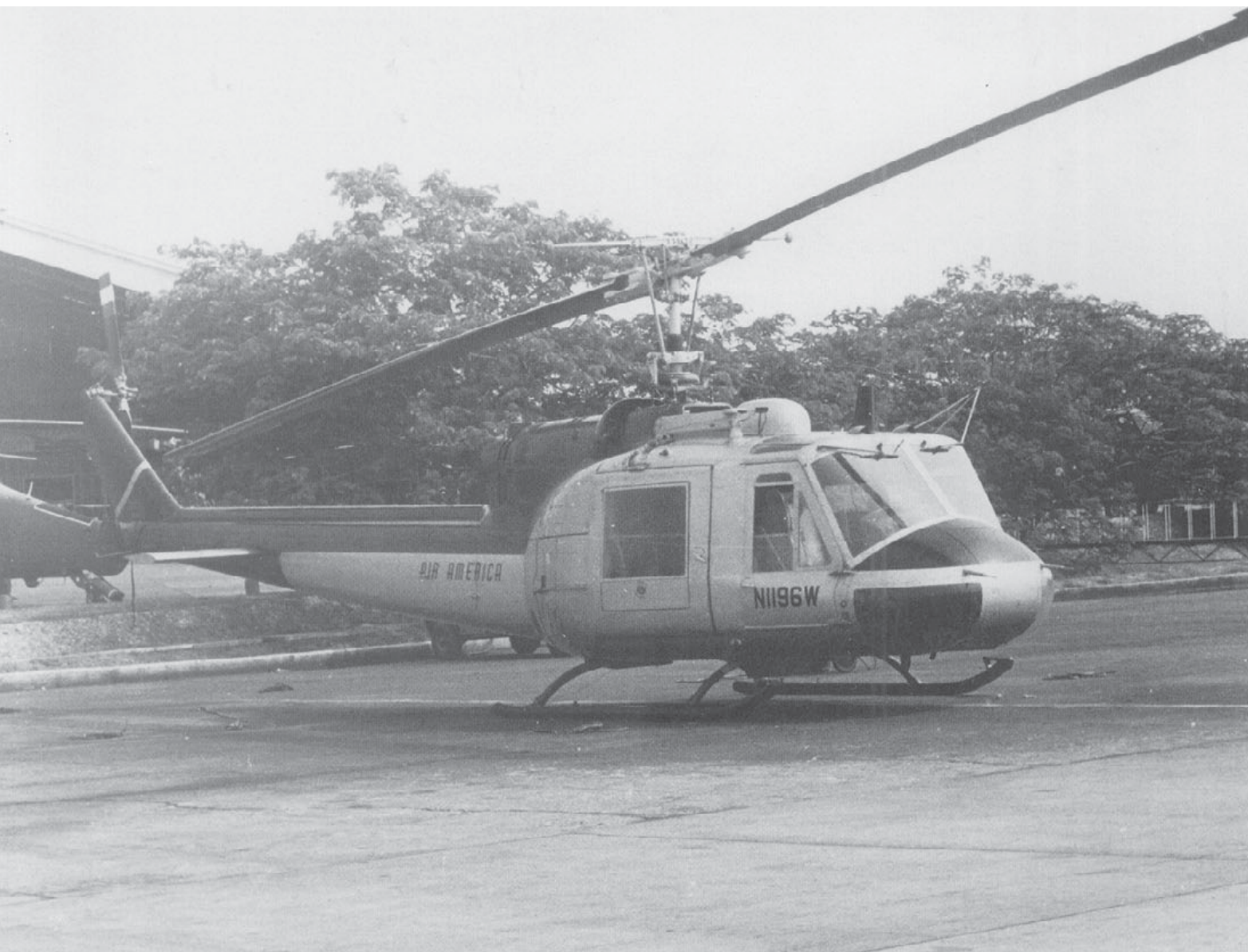
An Air America Bell 204B (N1196W) on the ramp at a RLA base. The Bell 204B was the civilian version of the military UH-1B Huey which could carry seven passengers. The larger Bell 205A, which could carry eleven passengers, saw greater use in Laos flown by Air America. (T.L. Arkansas)
