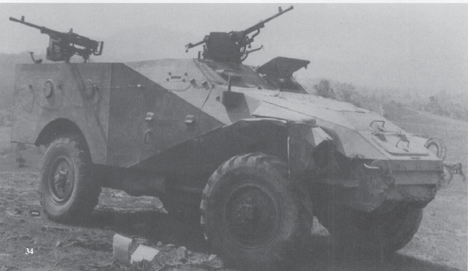
One of the Soviet-made BTR-40 armored personnel carriers captured during Operation KOU KIET. The vehicle was armed with a pair of 7.62mm medium machine guns, one mounted at the rear of the vehicle and one mounted at the front of the open personnel compartment. (Charles Campbell)
